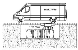
Coverage heights on installation in groundwater – the hatched area specifies the permissible immersion depth for the tank.
