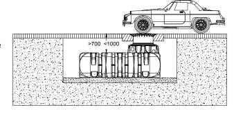
Coverage heights with cast telescopic dome shaft with cast iron lid or Begu (with cover class B respectively D - to be provided at construction site). Maximum load of the area used by passenger cars 3,5 to.
