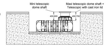
Maximum coverage heights with intermediate section and telescopic dome shaft.
