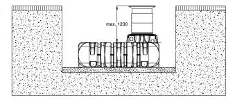
Coverage heights with cast telescopic dome shaft (class B) in areas used by passenger cars.
